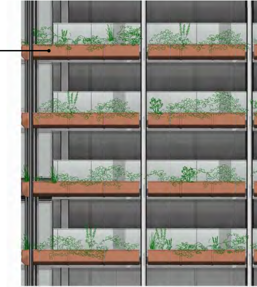
Zone 3 Hanging Garden Façade Elevation
